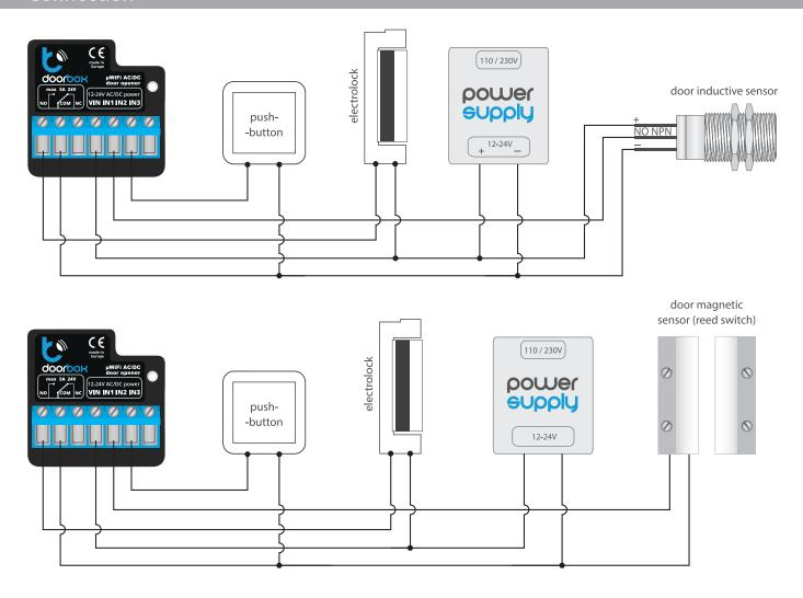
Start by connecting the +12V or +24V power wire (red or black with a white dotted line) to the VIN port and the ground (black) to the COM port.
