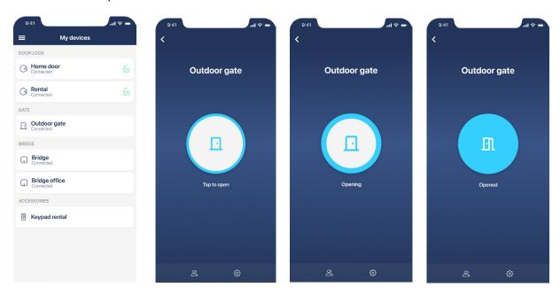
Tap the centre button to unlock the connected relay device.
