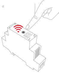
3. After releasing the button, the red LED will stay on for 2-5 seconds. During that time, the device must not be switched off or unplugged.
