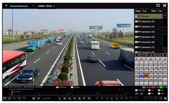
Figure 6-12 Interface of Playback by Time
