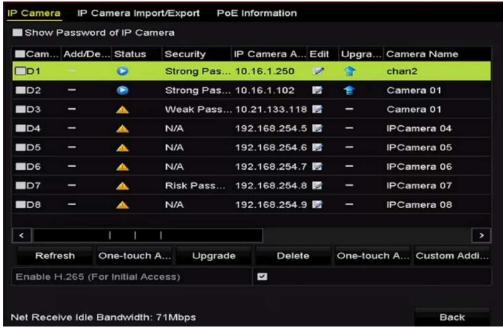
Figure 2-30 Adding IP Camera Interface
