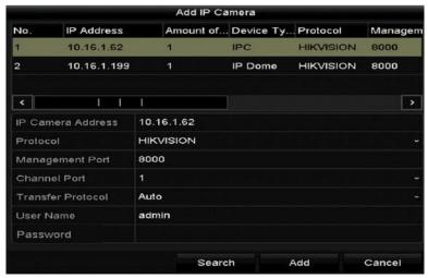
Figure 2-29 Quick Adding IP Camera Interface
