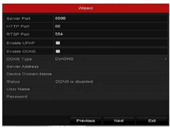
Figure 2-19 Advanced Network Parameters
