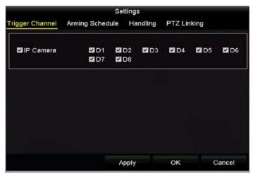
Figure 9-15 Set Trigger Cameras of POS
