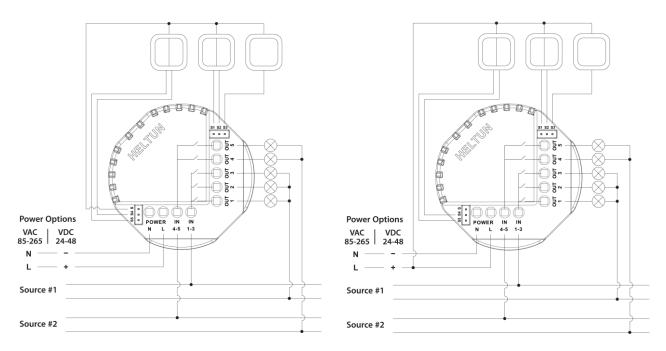
Figure 2: Power, Loads & External Switches Connection Diagram
