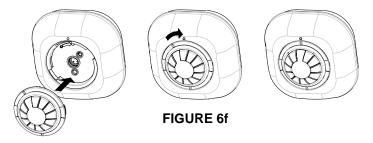
**Note:** To detect movements with detection coverage up to 360 degrees, simply reload the ceiling-lens cover without shading cap. No movements can be detected if the detector is reloaded with a shading cap which maintains 12 lens segments.
