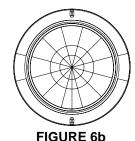
The shading cap is composed of 12 segments for limiting the detection coverage, and each segment covers detection angle of 30 degrees (FIGURE 6c). Follow the grooves on the cap, cut the cap to a suitable size and place it onto the ceiling-lens cover (FIGURE 6d). The remaining segments are used for blanking off an undesirable detection area.
