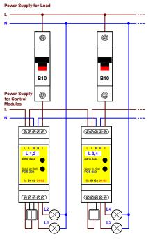
The descriptions of the screw terminals are printed on the adapter label. The letter "I" indicates input for powering the load devices. The "Q1" and "Q2" letters indicate the relays outputs.
