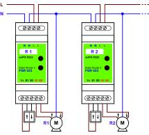
The descriptions of the screw terminals are printed on the adapter label. The "Q1" and "Q2" letters indicate the relays outputs.
